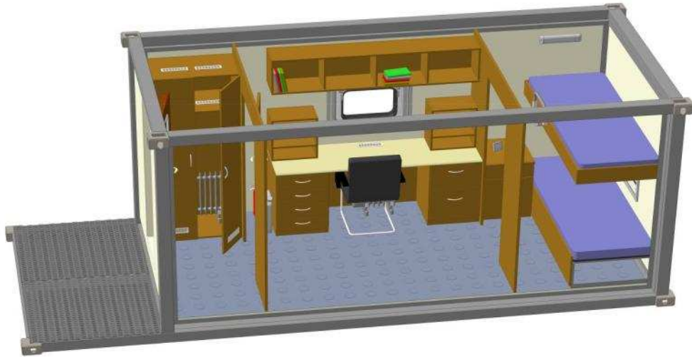
Figure 3 - Left section of the module. Right-side view From the entrance: a lobby, wardrobe with heating elements, lab workplace, compartment for recreation.
