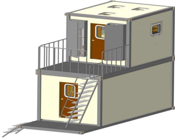
Figure 6 – General view of the laboratory & residential two-storey block module
